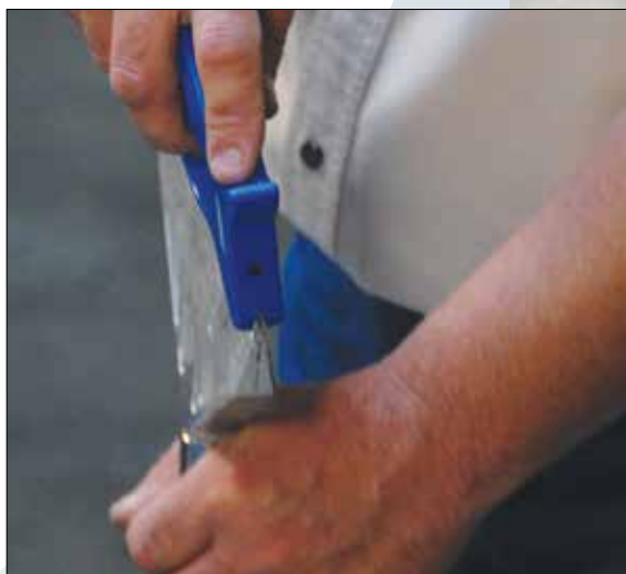
Resharpener of solid stainless steel scraper blades with a skirted design.
