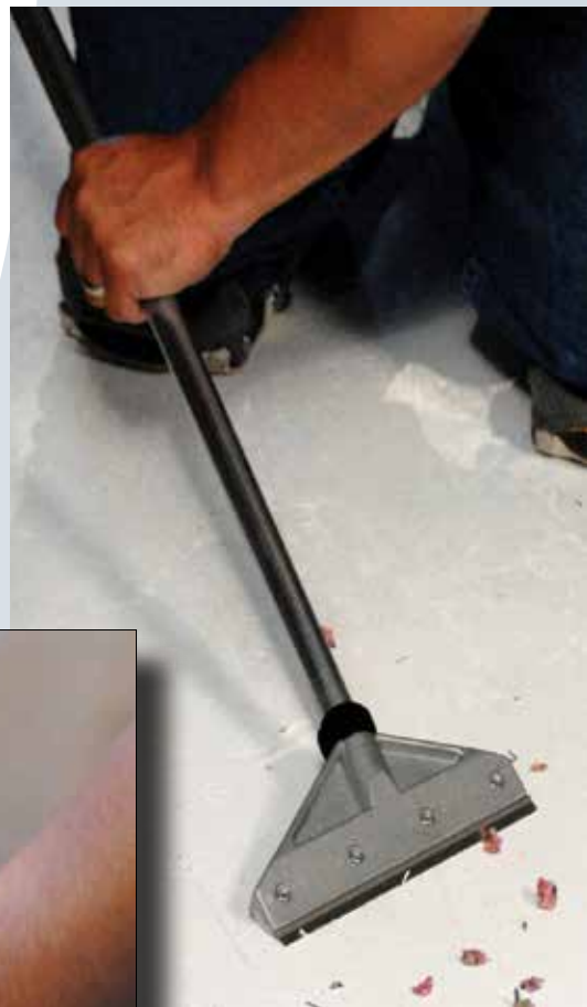
Solid stainless steel scraper blades with a skirted design allow for longer uninterrupted strokes.
